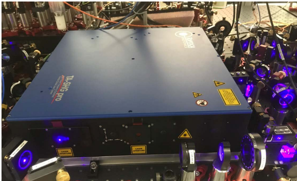
Commercial system (Toptica Photonics) to generate laser light at 421nm in our dysprosium laboratory.
