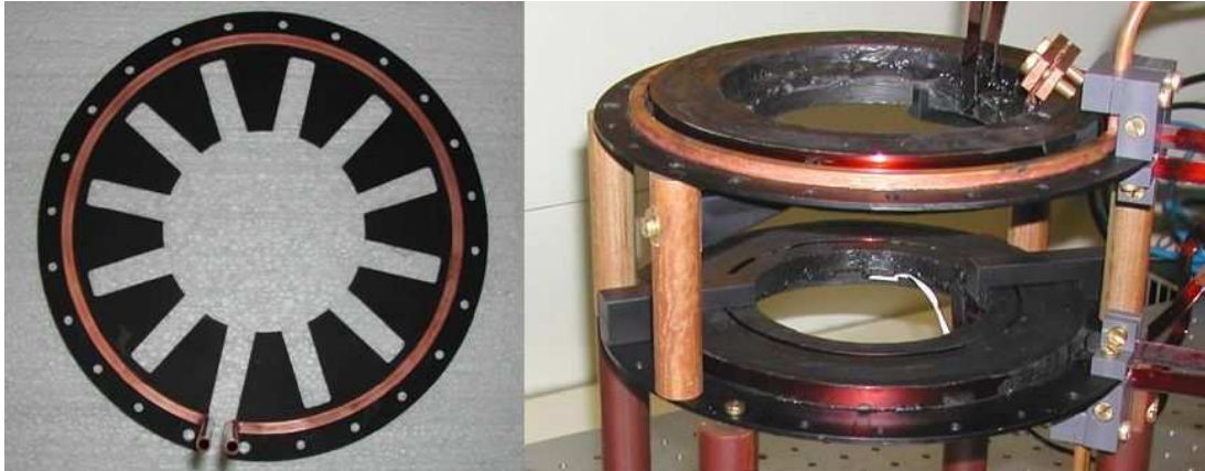
Figure 4.1: Left, the water-cooled mounting disc. Right, the assembled vertical coil construction.
