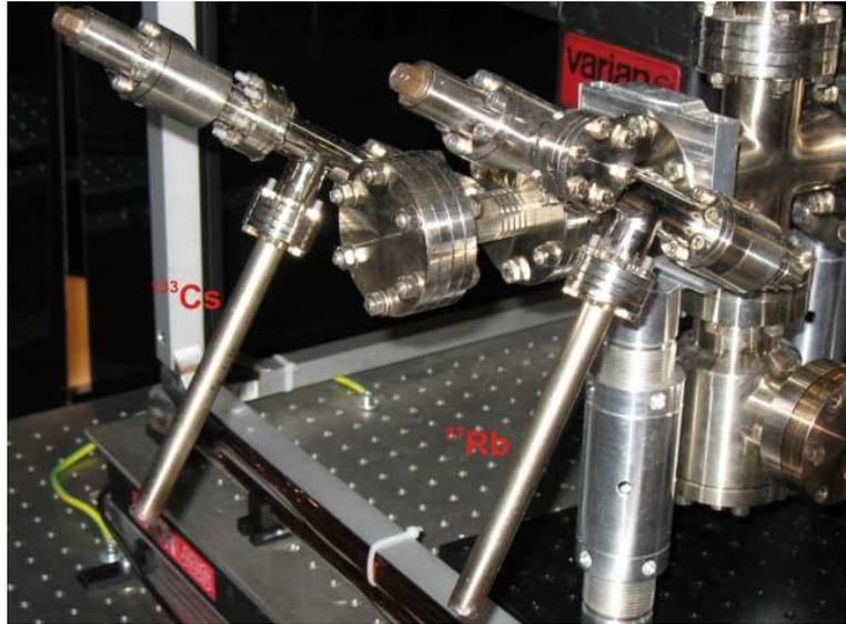
**Figure 3.2:** Photograph of the double-species oven. The different sections associated with the different species can be independently temperature controlled.
