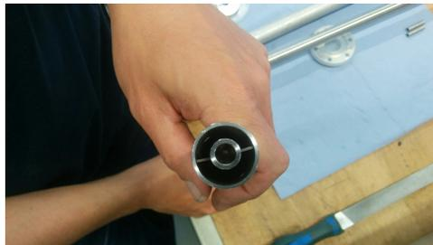
Figure A.6: Photograph of the double walled structure of the ZS with the inner vacuum tube and the two barriers.
