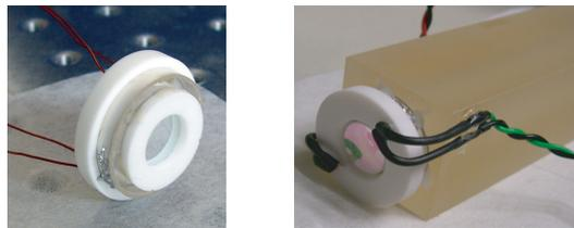
**Figure 4.6: Optical resonator piezos:** *left:* Nested piezo construction before gluing the outer piezo ring to the spacer. The large ceramic ring is attached to the outer piezo and supports the inner piezo. This in turn holds the smaller ceramic ring that the mirror is attached to. *right:* Zerodur spacer with piezos attached.
