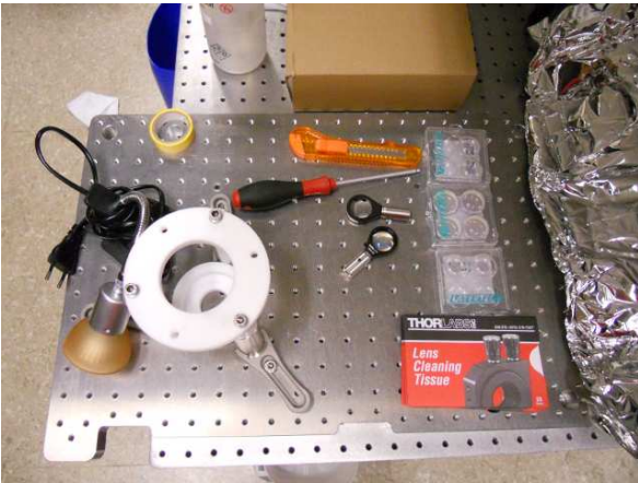
Figure A.8: Utensils used for optical contacting
